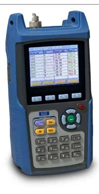
AE700 is a DWDM Channel Analyzer for the installation and maintenance of DWDM systems. The handheld unit is able to measure wavelengths in the c-band, which is from 1530 to 1565 nm. The AE700 also supports optical signal to ratio (OSNR) which is essential for verifying signal quality. The measurements can be displayed in both graphical or list formats.
